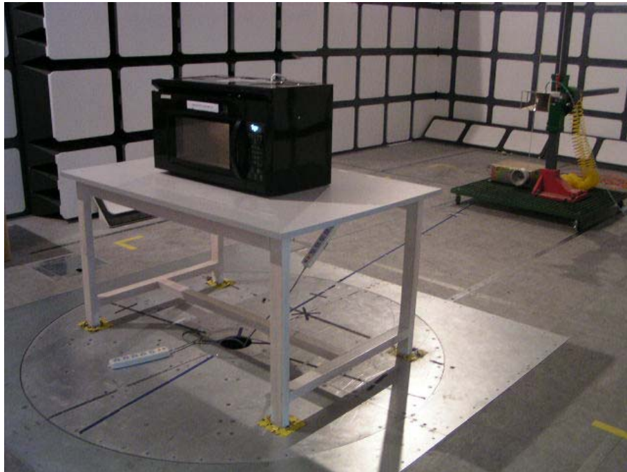
1000 MHz to 25GHz: Radiated Emissions-Front View
