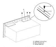
Loosen the 4 screws which fast the trim kit frame to the microwave oven, and set the 4 screws aside.
