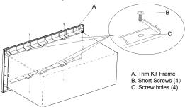
5. Release the 4 locating pins from locating holes, take out the trim kit frame, and set aside.
