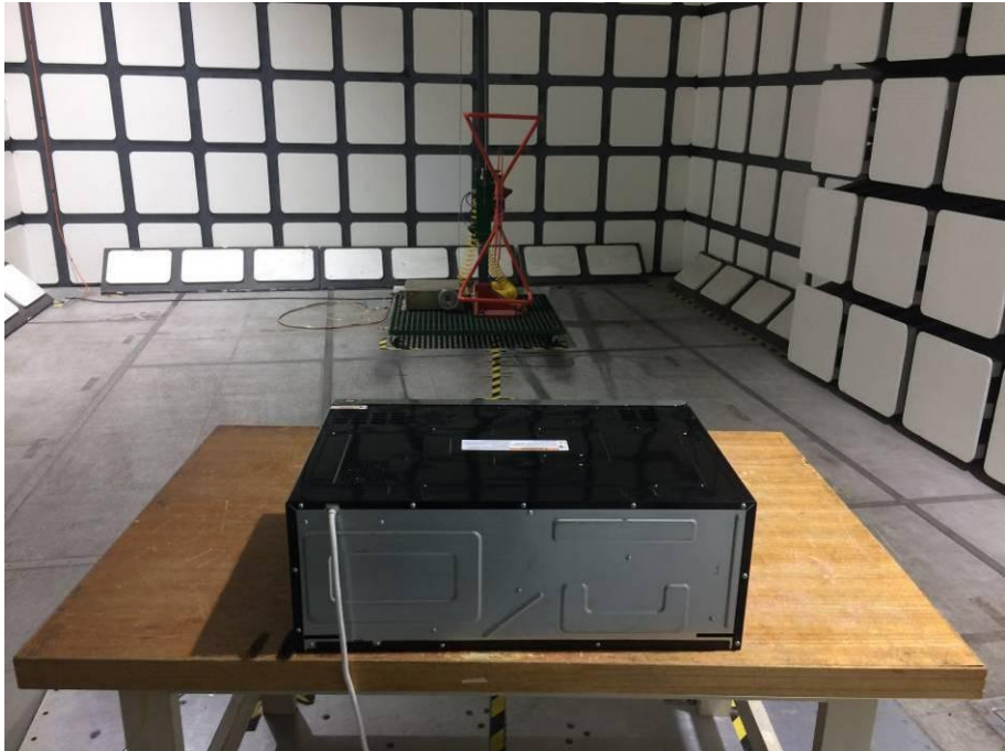
Radiated Emissions - Rear View (30 MHz – 1 GHz)
