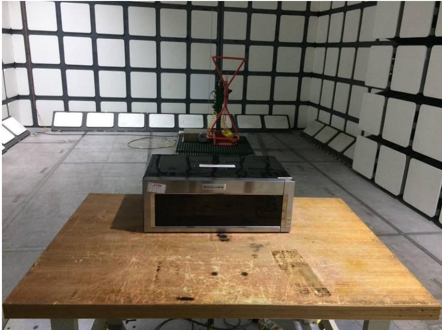
Radiated Emissions - Front View (30 MHz – 1 GHz)
