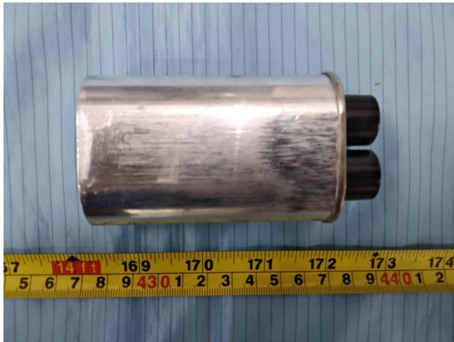
EUT – H.V. Capacitor Rear View
