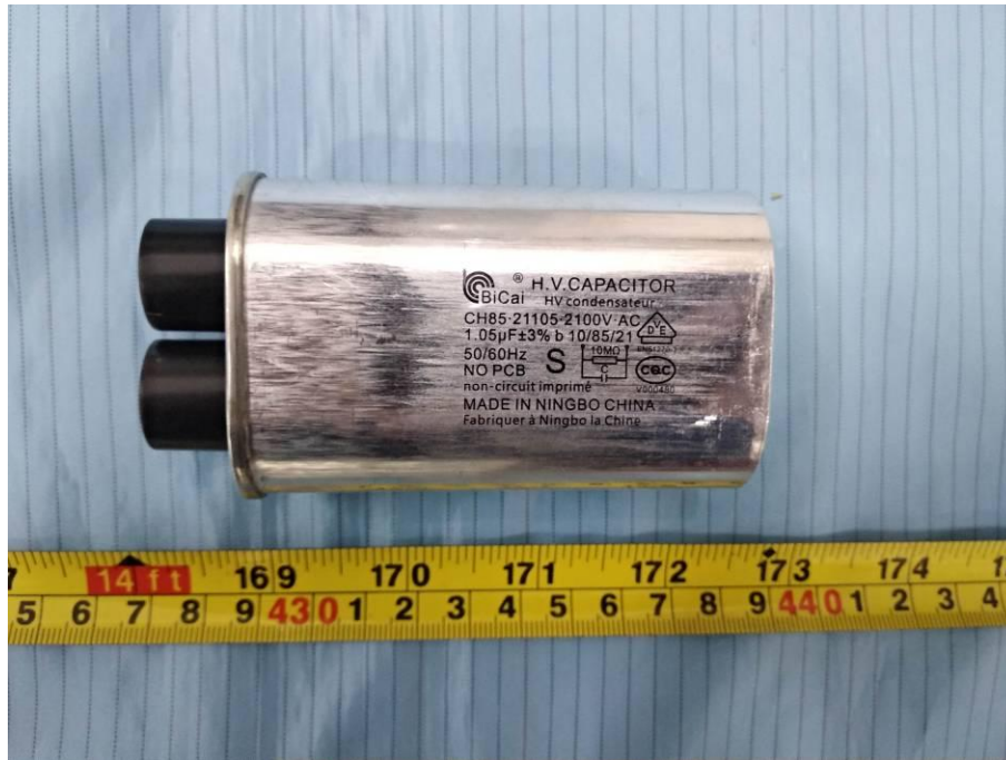
EUT – H.V. Capacitor Front View
