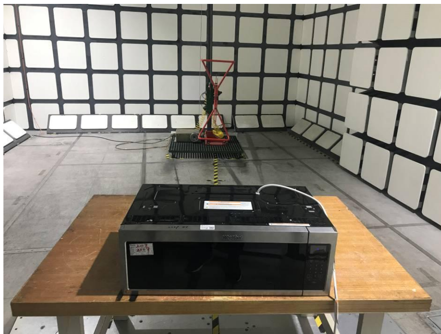
Radiated Emissions - Front View (30 MHz – 1 GHz)
