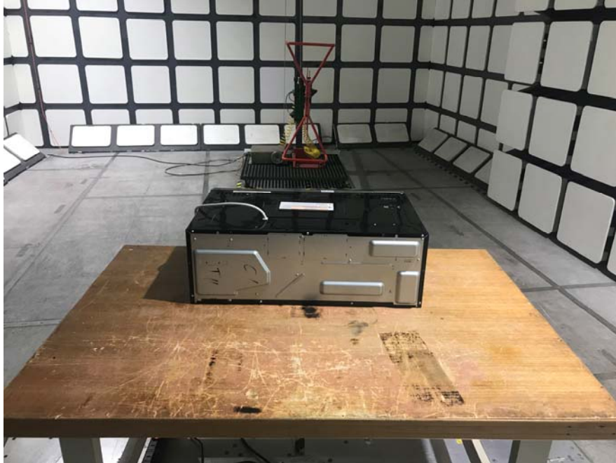
Radiated Emissions - Front View (30 MHz – 1 GHz)
