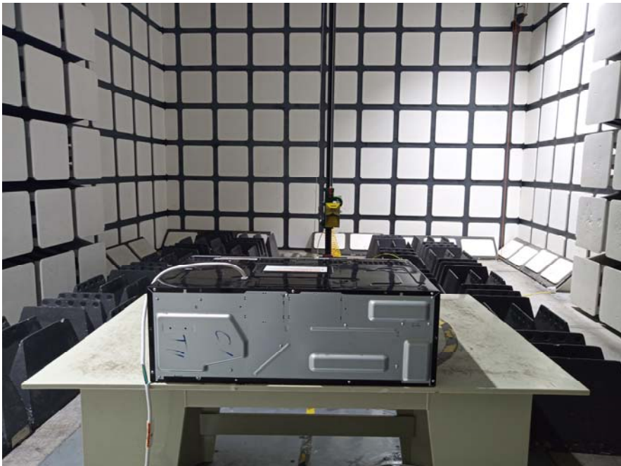
Radiated Emissions - Rear View (Above 1 GHz)
