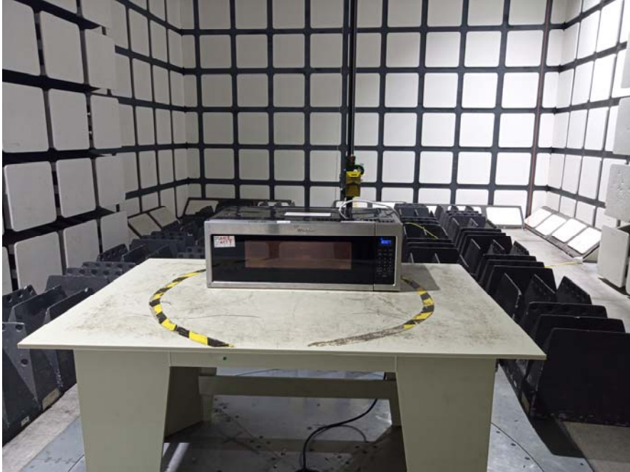
Radiated Emissions - Front View (Above 1 GHz)
