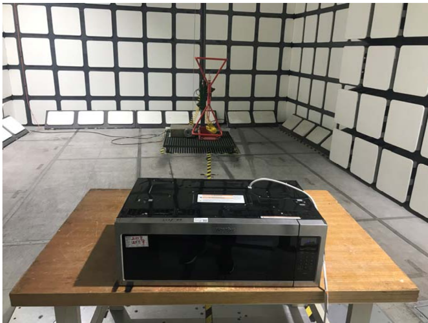
Radiated Emissions - Rear View (30 MHz – 1 GHz)
