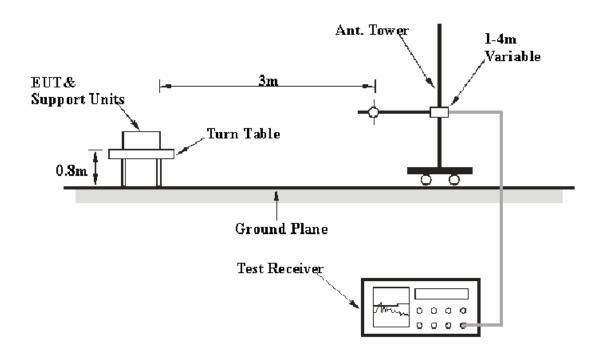
The radiated emission tests were performed in the 3 meters chamber test site, using the setup accordance with the FCC MP - 5. The specification used was the FCC part 18 limits.
