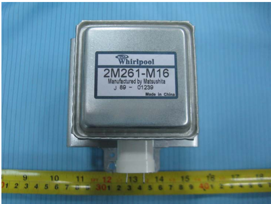
EUT – Magnetron View
