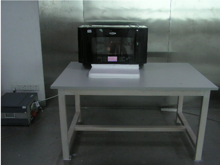
Conducted Emission–Front View
