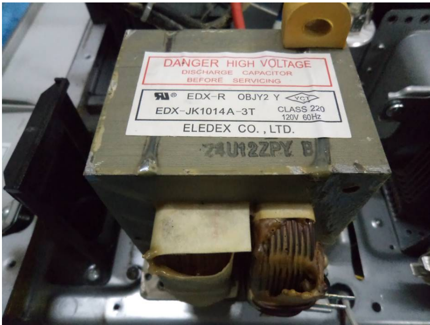
EUT – Power Transformer View
