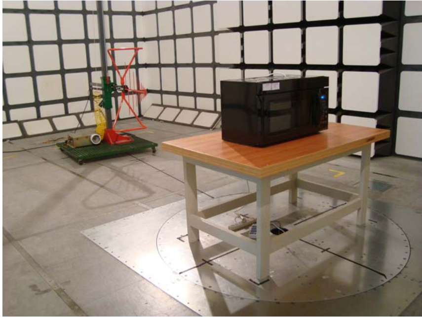
Radiated Emissions - Front View (30 MHz-1 GHz)
