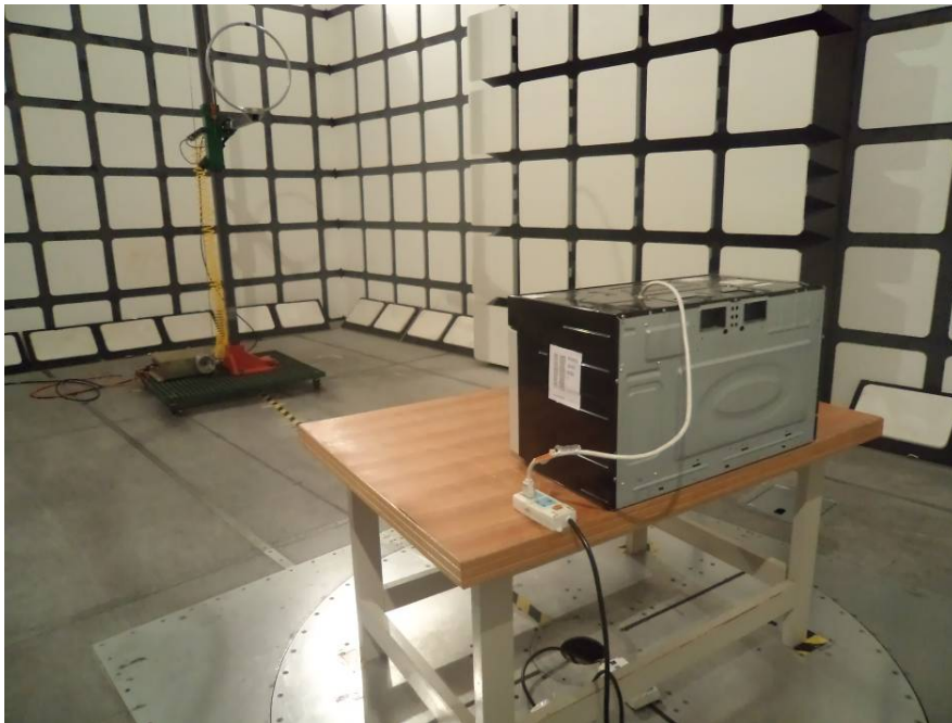
Radiated Emissions - Rear View (9 kHz – 30 MHz)
