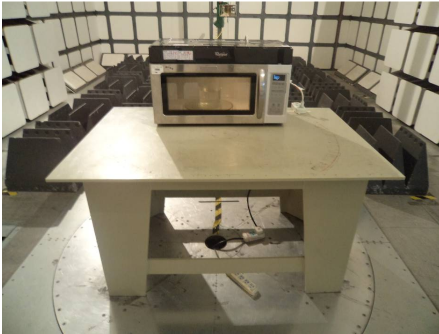
Radiated Emissions - Front View (Above 1 GHz)
