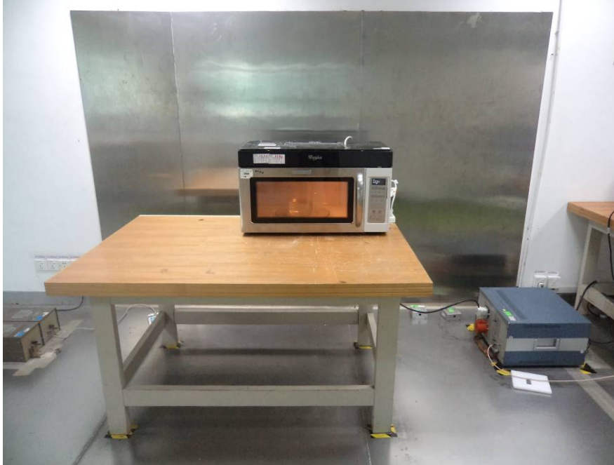
Conduction Emissions - Front View
