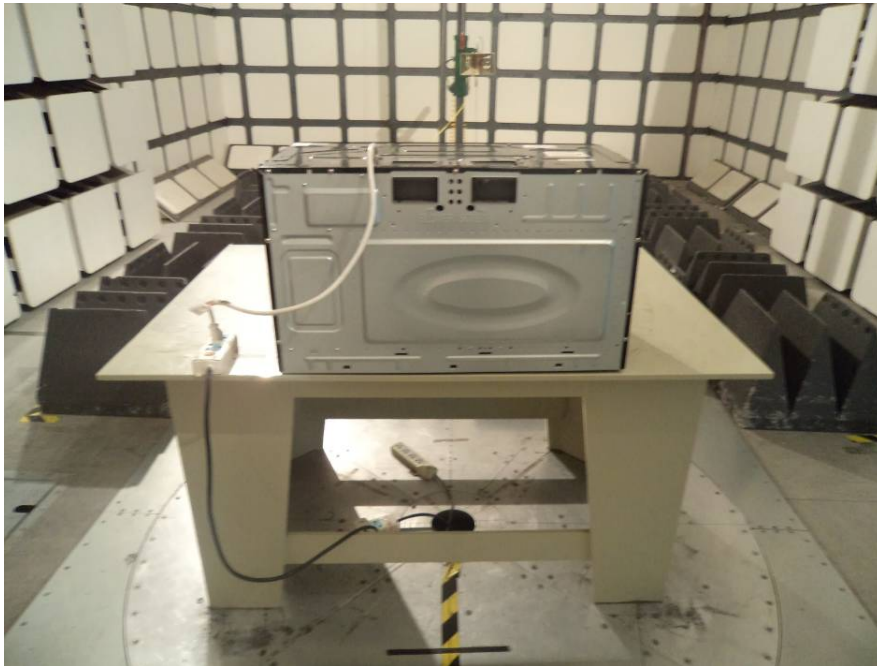
Radiated Emissions - Rear View (Above 1 GHz)
