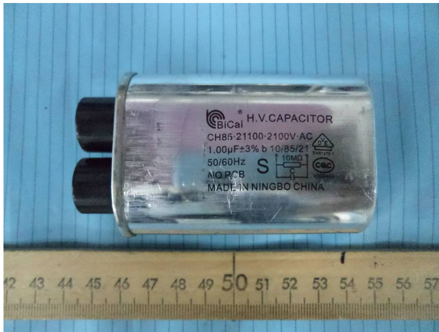
EUT – H.V. Capacitor View
