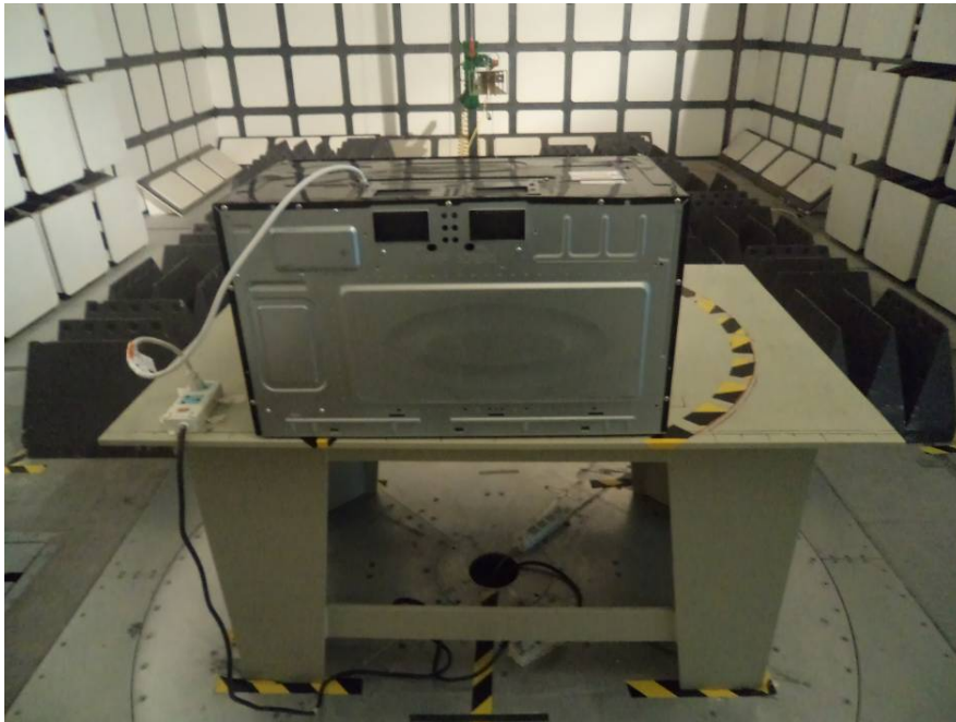
Radiated Emissions (1 GHz to 25 GHz) – Rear View
