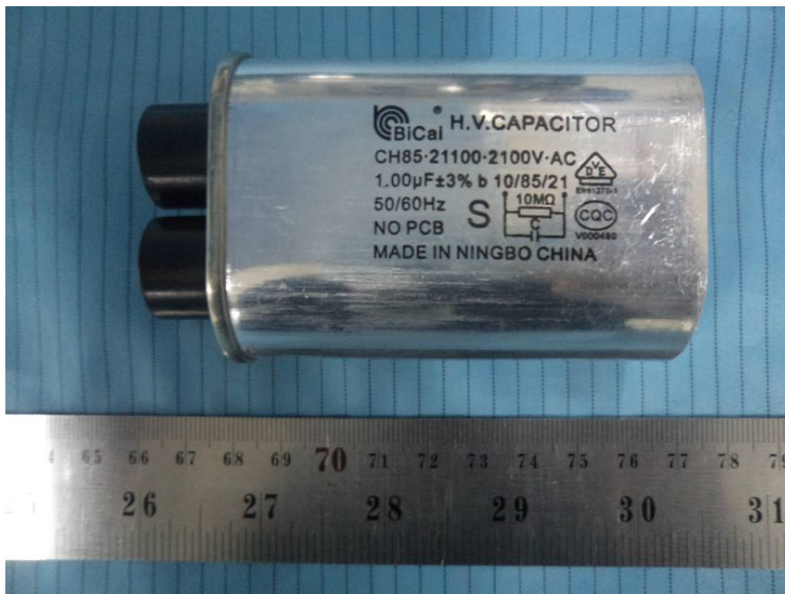
EUT – H.V. Capacitor Top View
