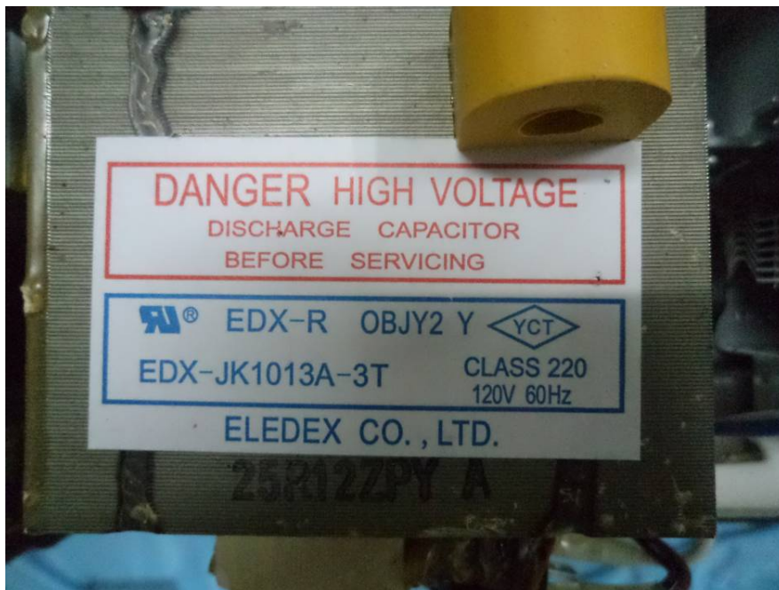
EUT – Transformer View
