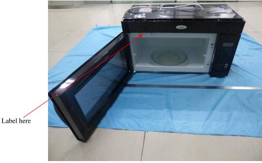
Specifications: Text is Black or white in color and is left justified. Labels are printed in indelible ink on permanent adhesive backing or silk-screened onto the EUT or shall be affixed at a conspicuous location on the EUT.
