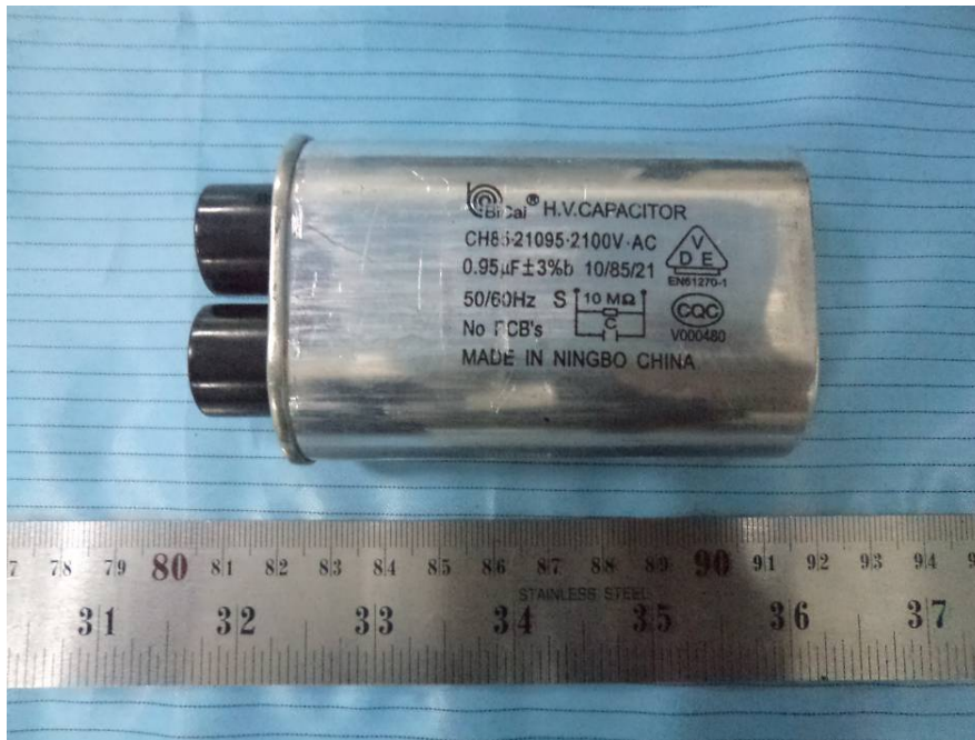
EUT – H.V. Capacitor View
