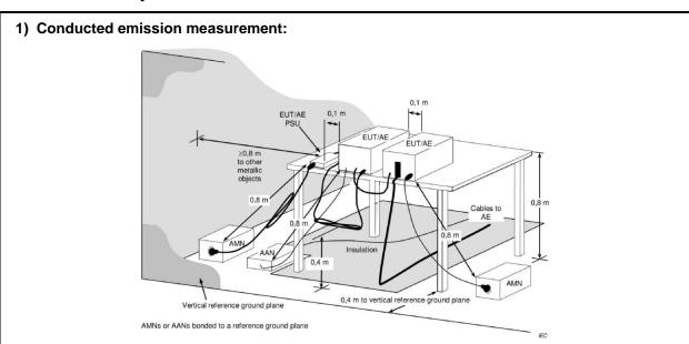
**Note:** The 0.8 m distance specified between EUT/AE/PSU and AMN/AAN, is applicable only to the EUT being measured. If the device is AE then it shall be >0.8 m.
