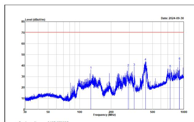
Project No. : 2405W25903E Test Mode : Microwave Test Voltage : AC 120V/60Hz
