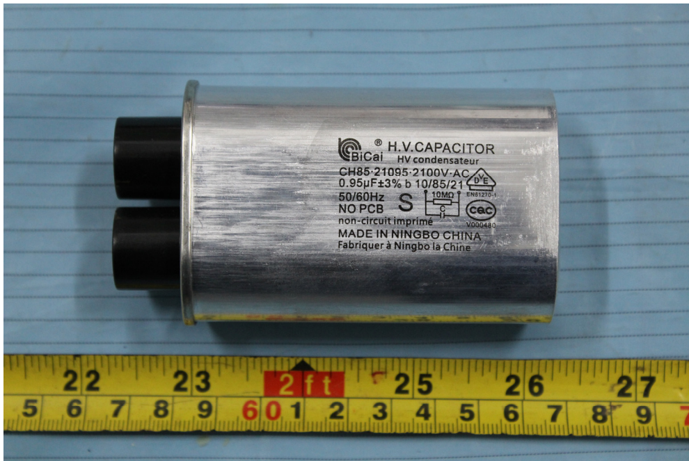
EUT – H.V. Capacitor View
