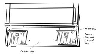
Clean the grease filter monthly, or replace with new grease filter if necessary.
