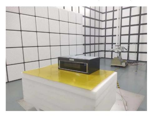
**Radiated Emissions Test View (Above 1GHz)**
