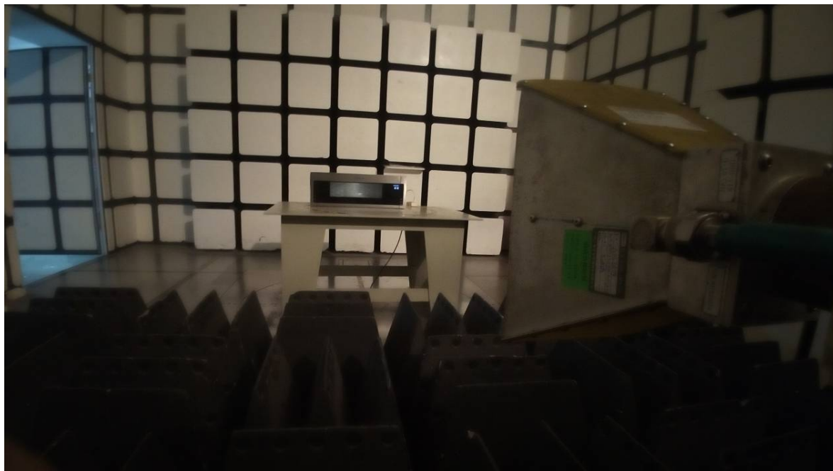
Radiated Emissions - Front View (Above 1 GHz)
