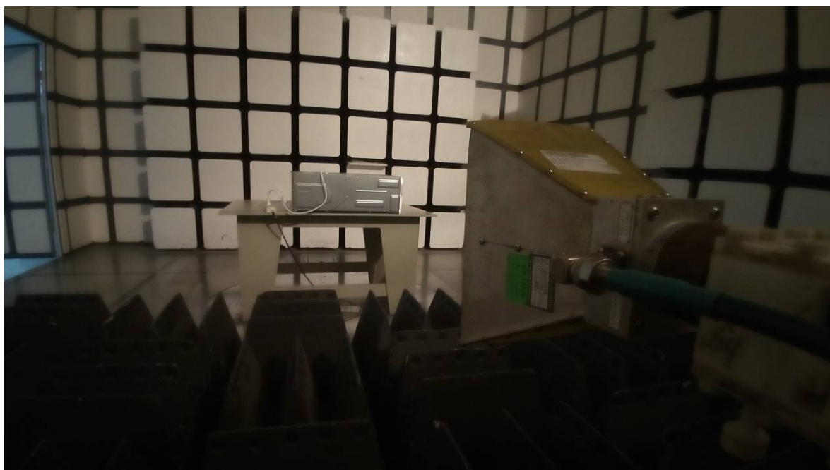
Radiated Emissions - Rear View (Above 1 GHz)
