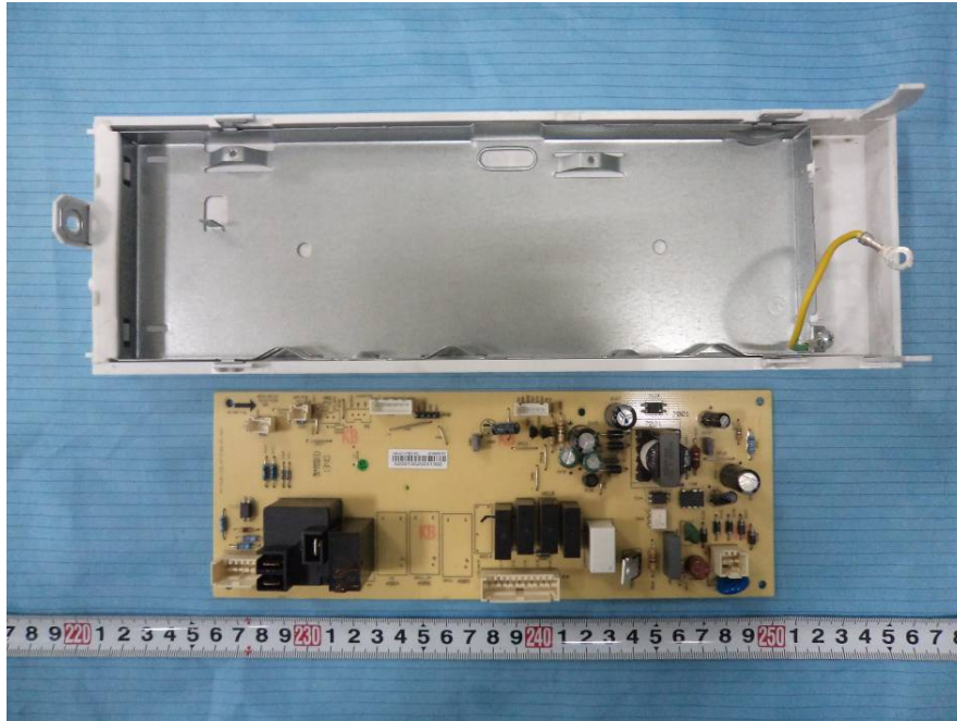
EUT –Control Panel Cover off View
