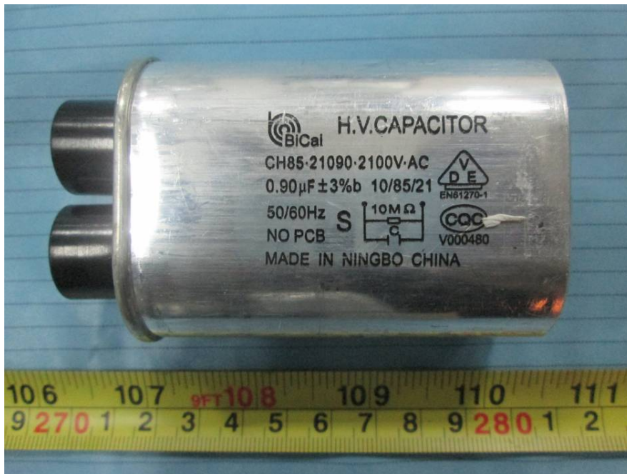
EUT – H.V. Capacitor View
