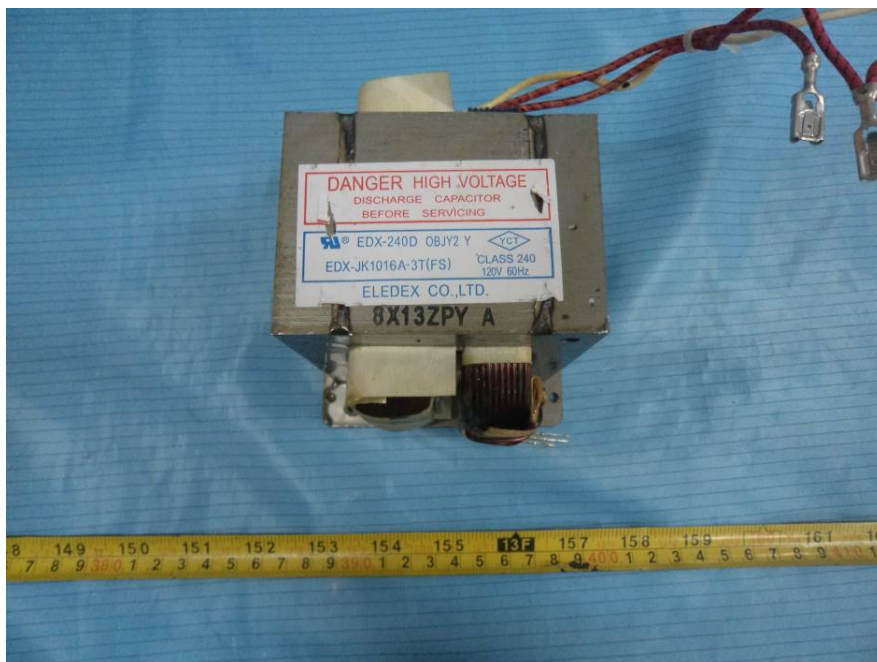
EUT – Power Transformer View
