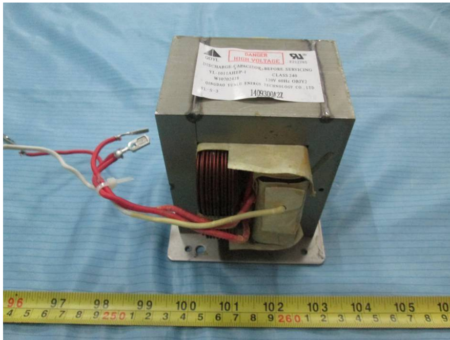
EUT –High voltage transformer
