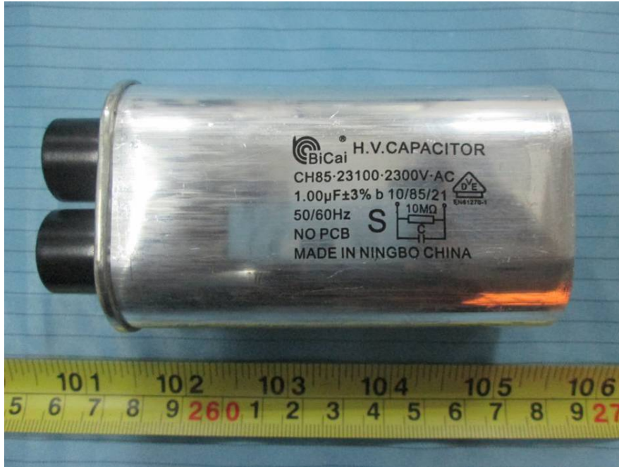
EUT – H.V. Capacitor View
