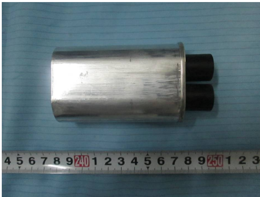
EUT – H.V. Capacitor Rear View
