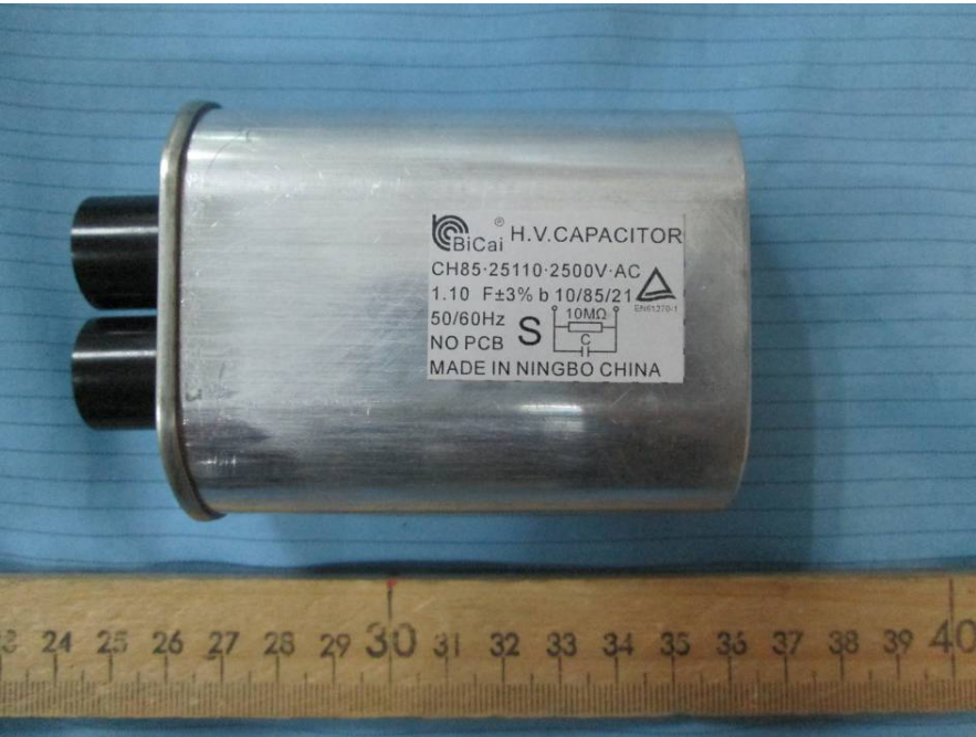
EUT – H.V. Capacitor View
