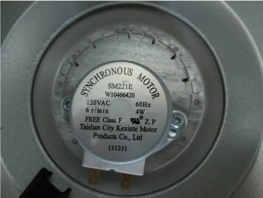
EUT – Synchronous Motor View
