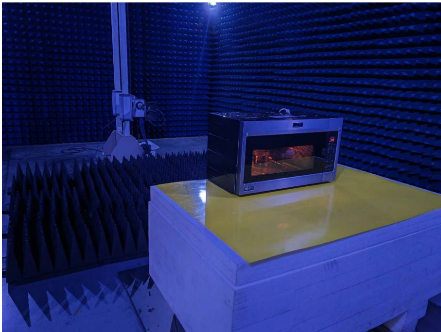
Photo of Radiated Emission Measurement Above 1GHz
