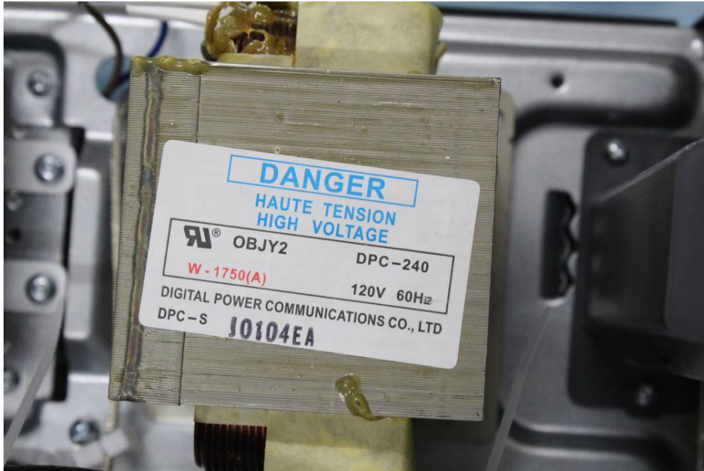
EUT – Transformer View
