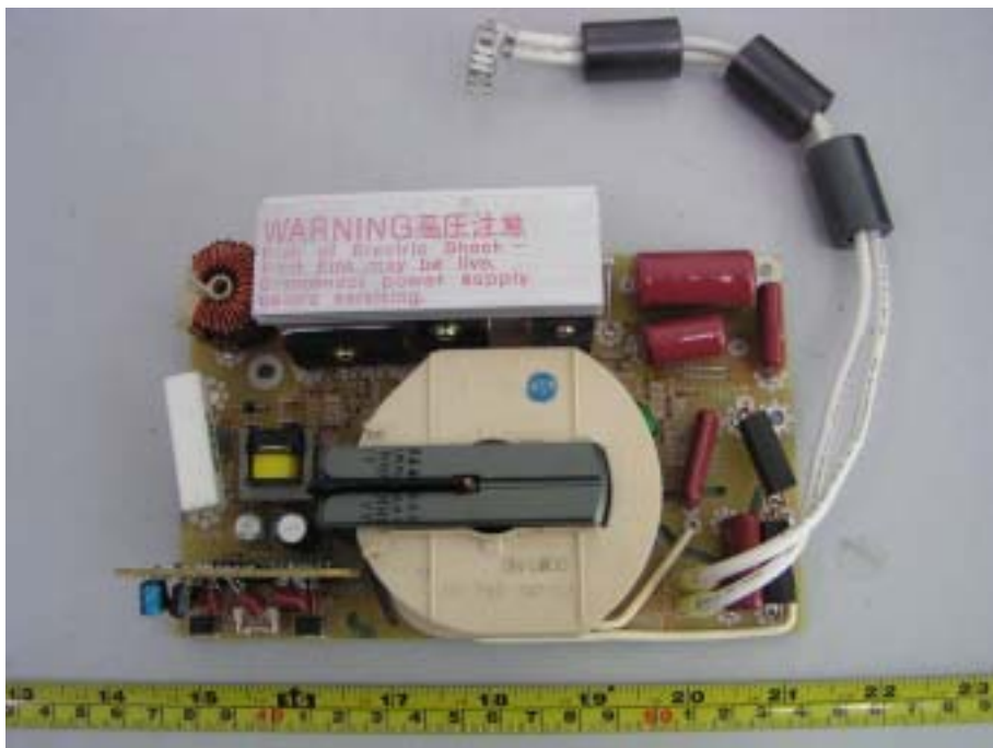
EUT – Transformer View
