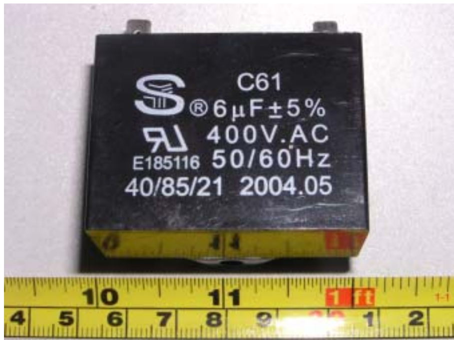
EUT – Filter Capacitor 1 View
