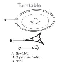
**NOTE:** By touching the Turntable keypad, it is possible to switch the turntable on and off during manual cooking cycles. This is helpful when cooking with plates that are bigger than the turntable or when cooking with plates side by side.
