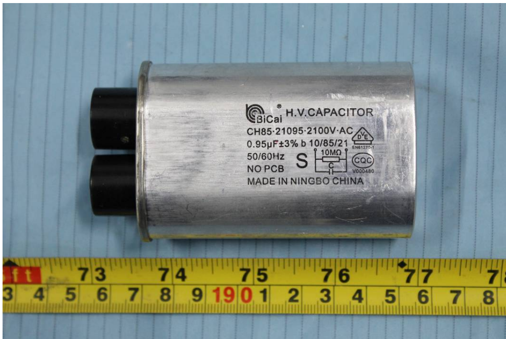
EUT –High Voltage Capacitor View
