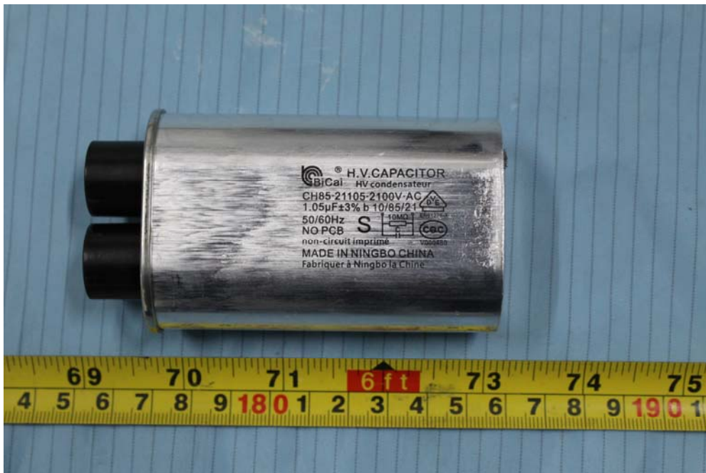
EUT –High Voltage Capacitor View
