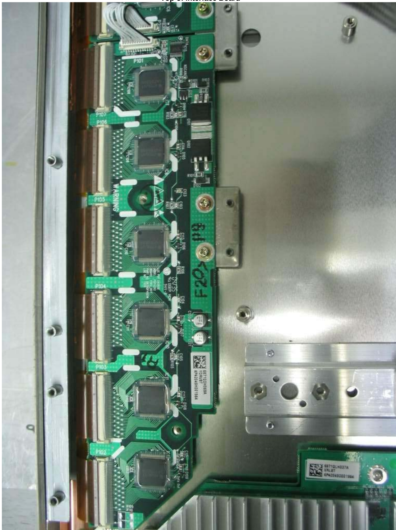
Top of interface Board
