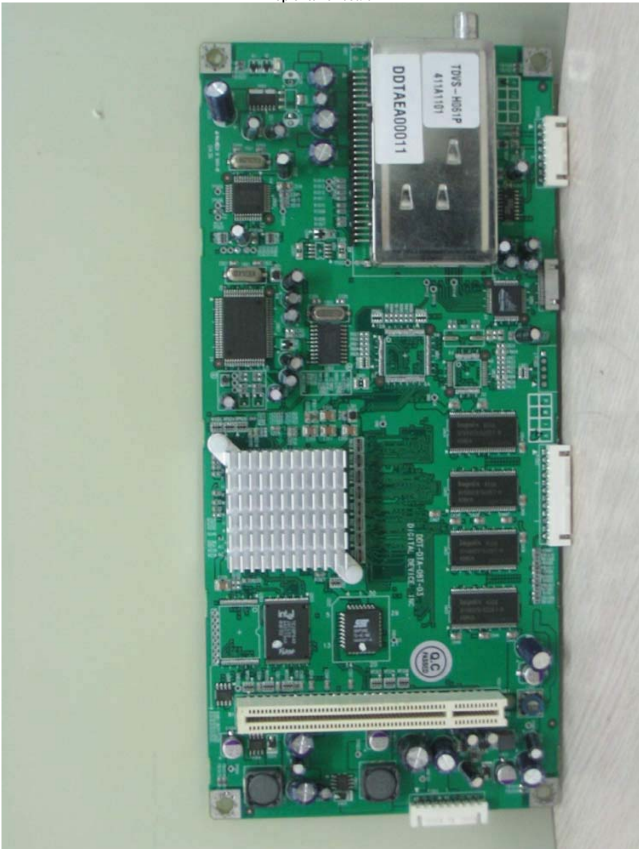
Top of tuner board
