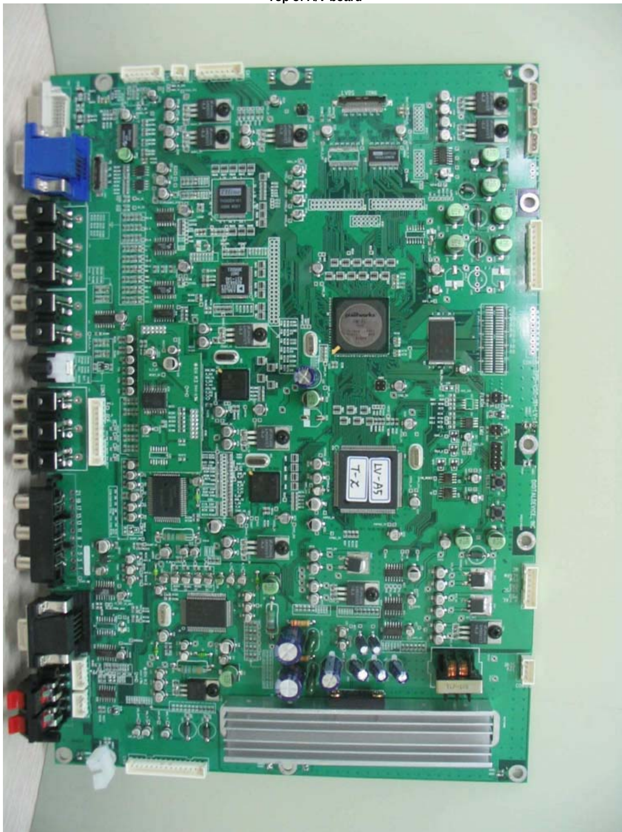
Top of A/V board
