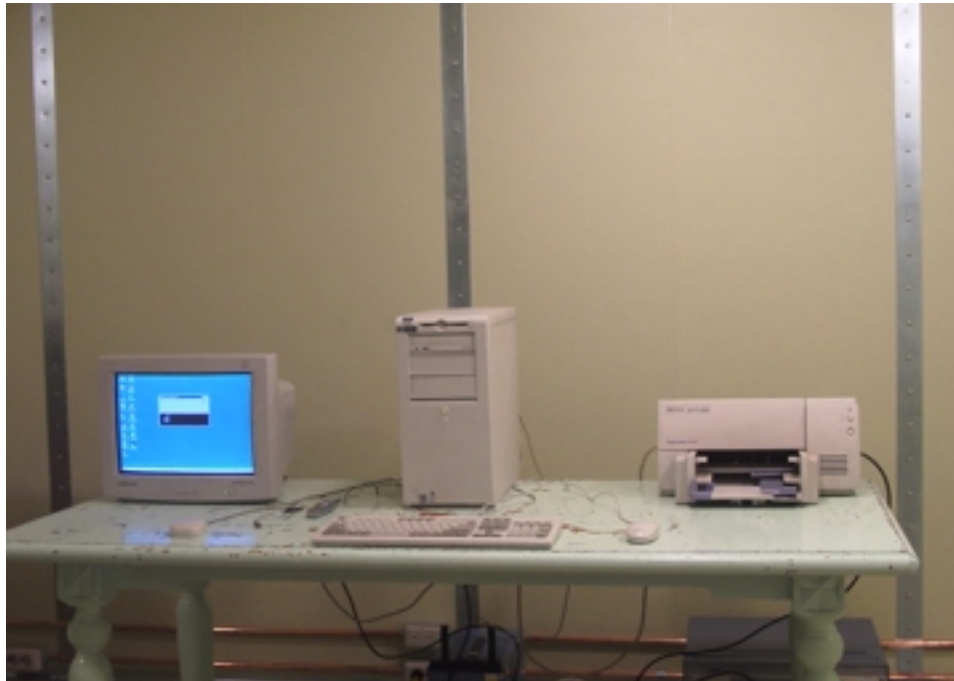
Photograph 2 : Setup for Conducted Emissions
