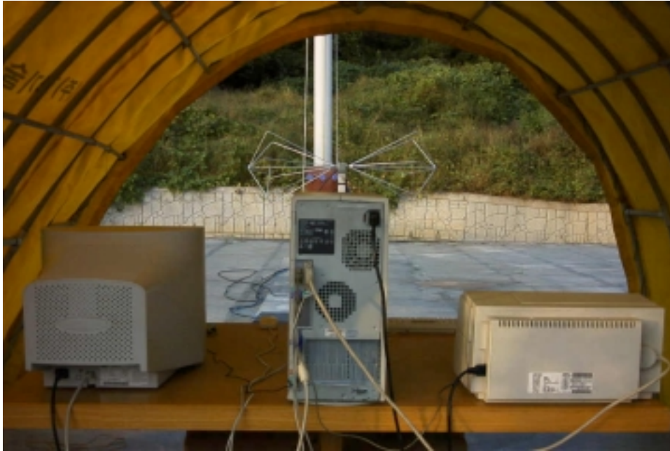
Photograph 1 : Setup for radiated Emissions
