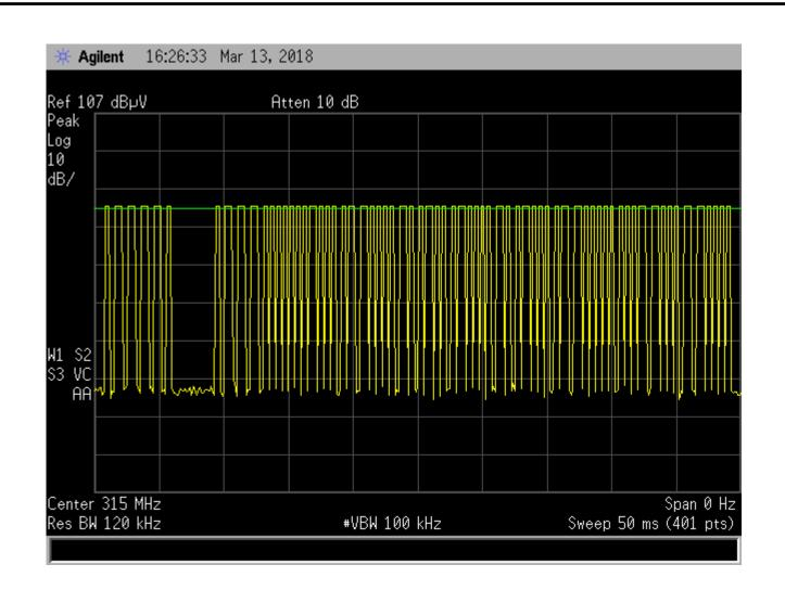
Test Method: FCC Part 15.231(b), Duty Cycle Determination Notes: Number of Pulses = 46 @ 0.2375 ms; 17 @ 0.4875 ms
