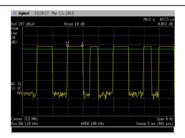
Test Method: FCC Part 15.231(b), Duty Cycle Determination Notes: Pulse width on time =  $487.5 \ \mu S$
