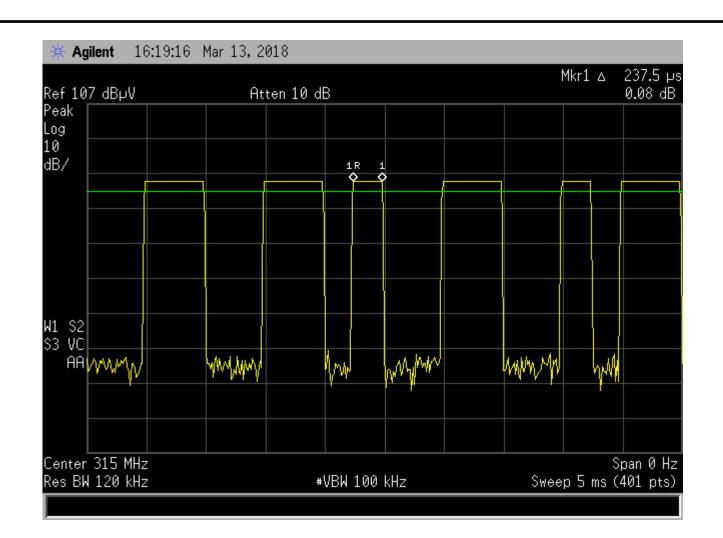
Test Method: FCC Part 15.231(b), Duty Cycle Determination Notes: Pulse width on time =  $237.5 \ \mu S$
