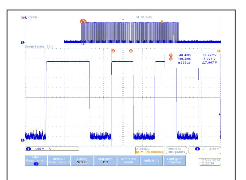
Test Method: FCC Part 15.231(b)(2), Duty Cycle Determination IC RSS-210 A1.1.2(2) Pulsed Operation Notes: Pulse width 2 = 0.222 ms
