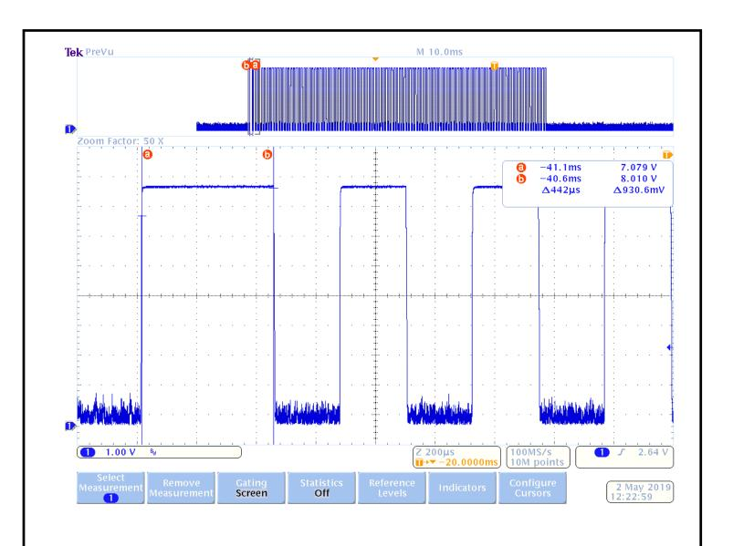
Test Method: FCC Part 15.231(b)(2), Duty Cycle Determination IC RSS-210 A1.1.2(2) Pulsed Operation Notes: Pulse width  $1=0.442\ ms$
