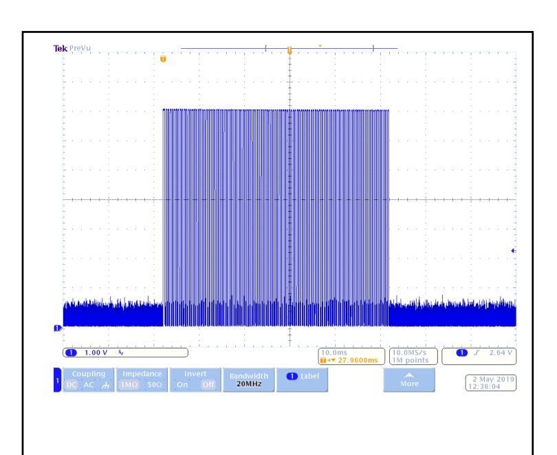
Test Method: FCC Part 15.231(b)(2), Duty Cycle Determination IC RSS-210 A1.1.2(2) Pulsed Operation Notes: Number of Pulses = 1 @ 0.442 ms; 111 @ 0.222 ms Averaging Interval = 49.6 ms; Duty Cycle = 50.6%
