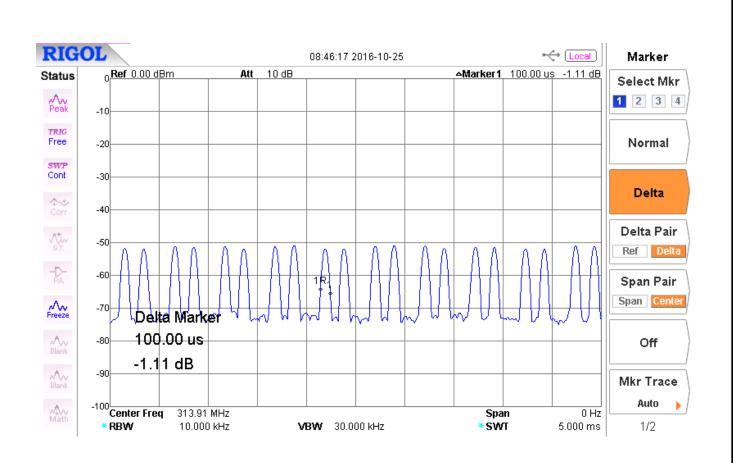
Test Method: FCC Part 15.231(b), Duty Cycle Determination
