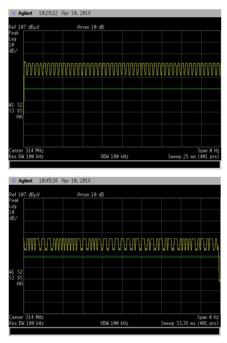
Test Method: FCC Part 15.231(b), Duty Cycle Determination
