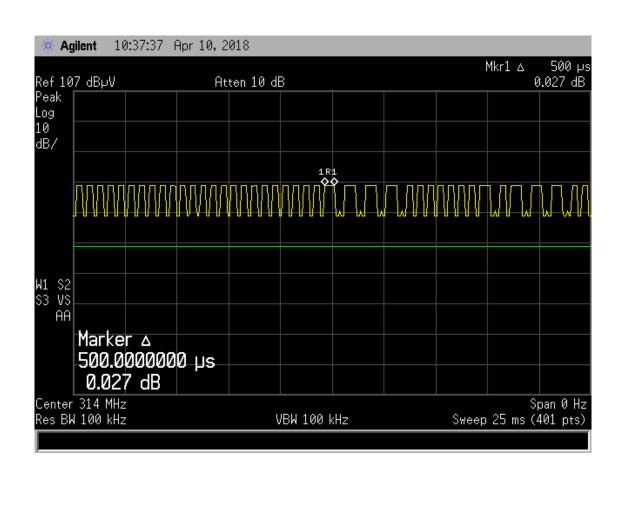
Test Method: FCC Part 15.231(b), Duty Cycle Determination Notes: Pulse width on time =  $500 \ \mu S$
