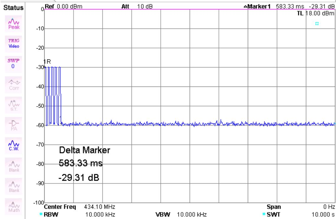
**Test Method: FCC Part 15.231(a)(1), Transmitter Deactivation Time**
