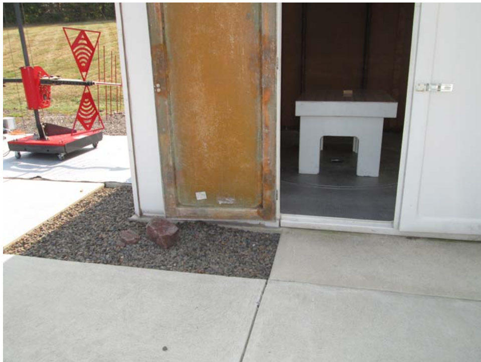
Vertical Antenna Polarization, Below 1 GHz
