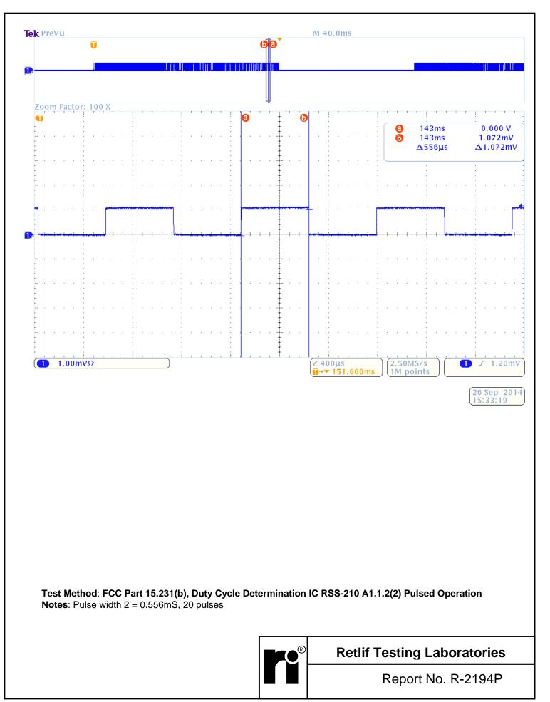
Pulse Train = T = 261 mS Averaging Interval = A1 = lesser of T and 100 mS Number of different Pulse Widths = N = 2 Pulse Width 1 = 0.276 mS Pulse Width N = 0.556 mS Number of PW1 pulses = #P1 = 175Number of PWN pulses = #PN = 20Ton = (PW1 \* #P1) + (PWN \* #PN) = 48.3 + 11.12 = 59.42 Ms Duty Cycle = Ton / A1 = 0.5942
