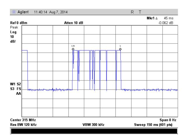
Test Method: FCC Part 15.231(b), Duty Cycle Determination Notes: Measurement of cycle time = 45.0 ms
