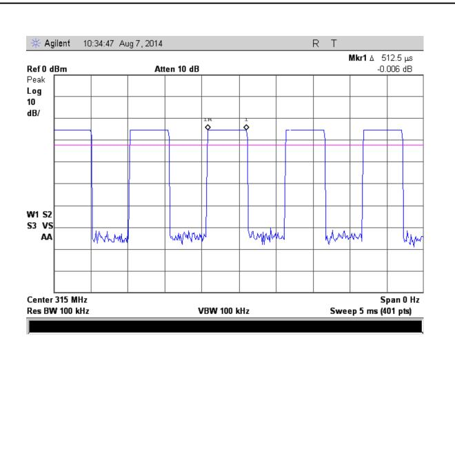
Test Method: FCC Part 15.231(b), Duty Cycle Determination IC RSS-210 A1.1.2(2) Pulsed Operation Notes: Pulse width 1 = 512.5 us; 82 Pulses
