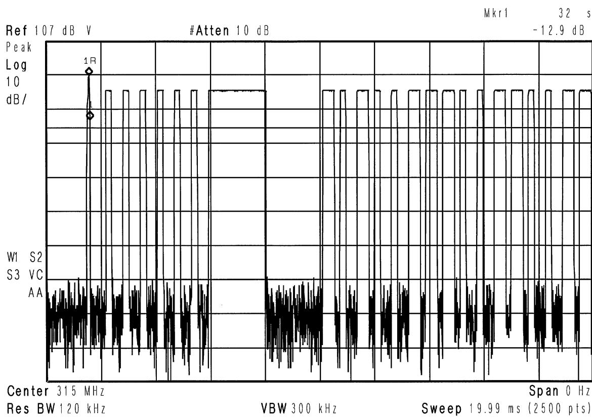
**Test Method: FCC Part 15.231(b), Duty Cycle Determination IC RSS-210 A1.1.2(2) Pulsed Operation**
