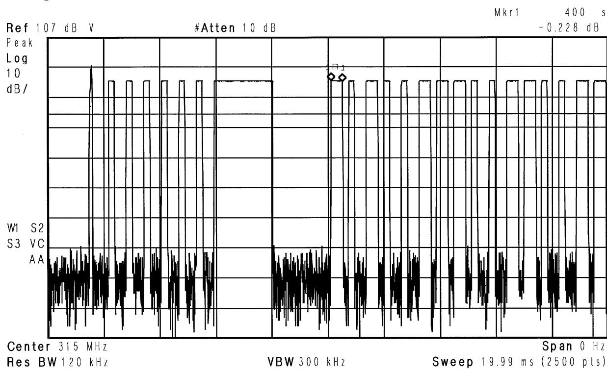
**Test Method: FCC Part 15.231(b), Duty Cycle Determination IC RSS-210 A1.1.2(2) Pulsed Operation**
