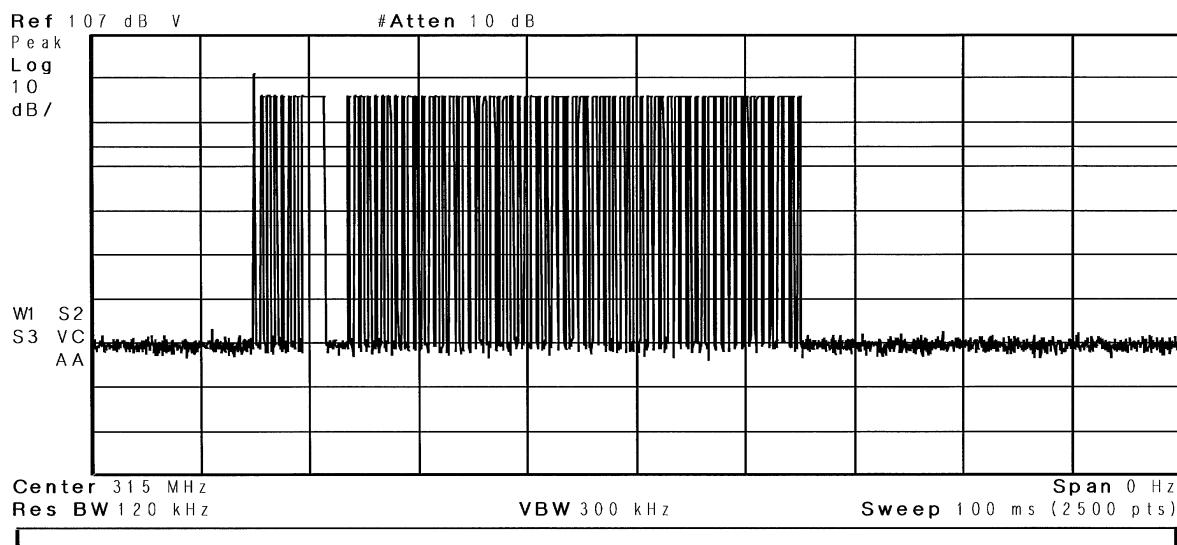
**Test Method: FCC Part 15.231(b), Duty Cycle Determination IC RSS-210 A1.1.2(2) Pulsed Operation**
