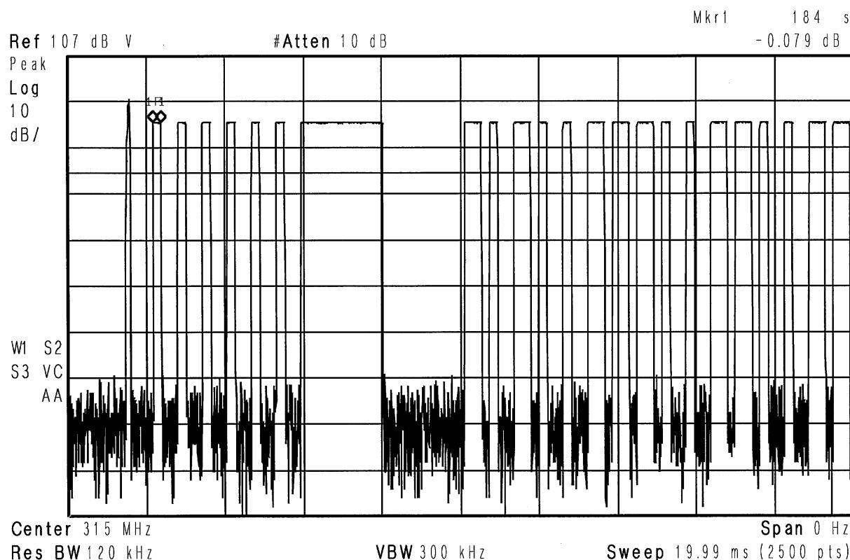
**Test Method: FCC Part 15.231(b), Duty Cycle Determination IC RSS-210 A1.1.2(2) Pulsed Operation**
