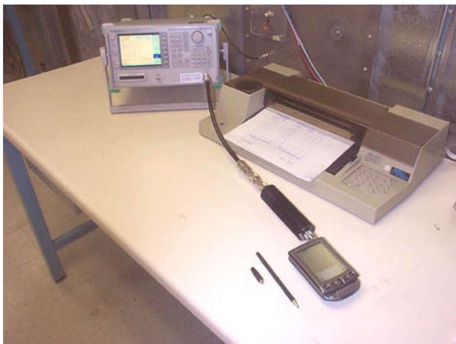
Testing Spurious Radiation from Transmitter at Antenna Port Palm attached to DUALWAVE M Wireless Modem
