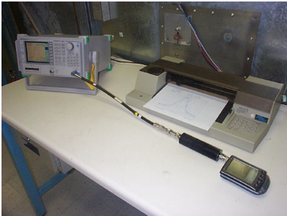
Testing Occupied Bandwidth on Palm and DUALWAVE M Wireless Modem
