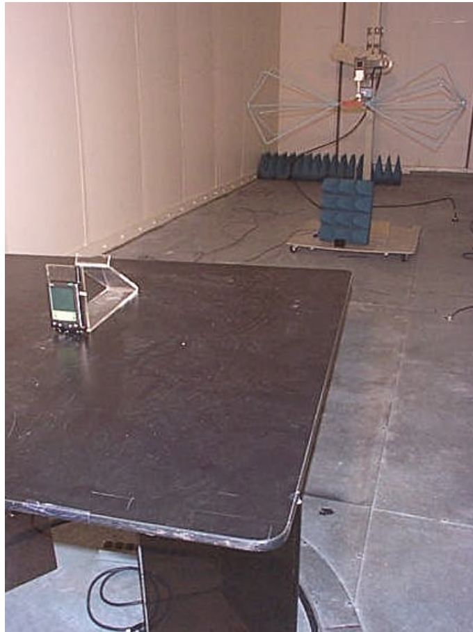
Palm and WaveNet DUALWAVE M Wireless modem Testing for Spurious Emissions from Transmitter Frequency Range: 30 MHz – 200 MHz
