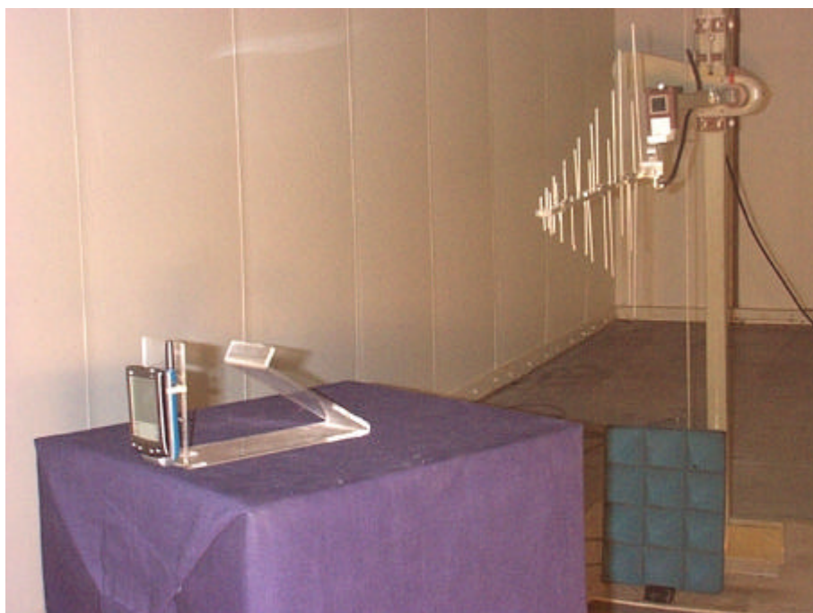
ERP Testing – Vertical Position Wireless Modem attached to Palm
